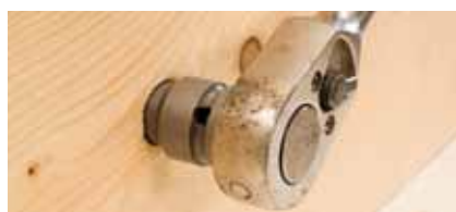
6. Release insertion sleeve with ratchet.
