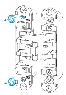
Gasket pressure adjustment +/- 1 mm
